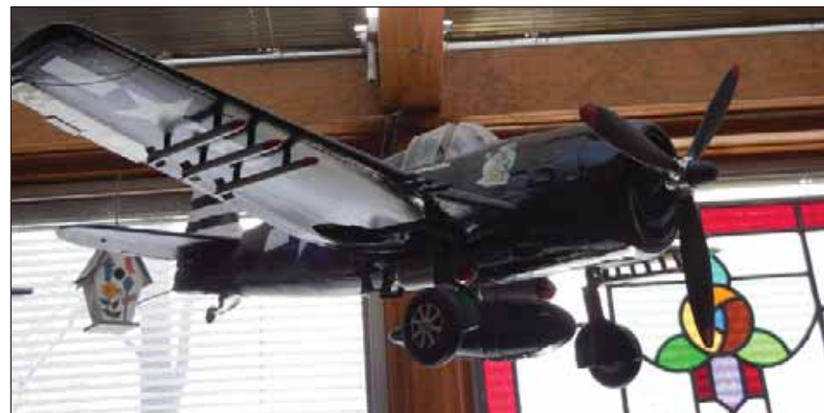
Muirhead built this model replica of his Hellcat fighter-bomber. Note machine guns at front of wings, missiles under the wings and bombs on either side of the gas tank under the fuselage.
